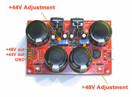
Actually, both outputs can be adjusted to whatever voltage you need... 45V, 46V, etc.
